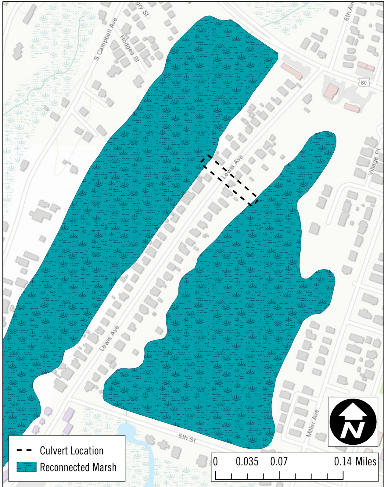
Figure 5.9. Potential location of the underground culvert to reconnect both marshes around Lewis St.
