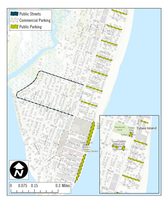
Figure 5.15. Proposed permeable paver locations that include both commercial and public property.
